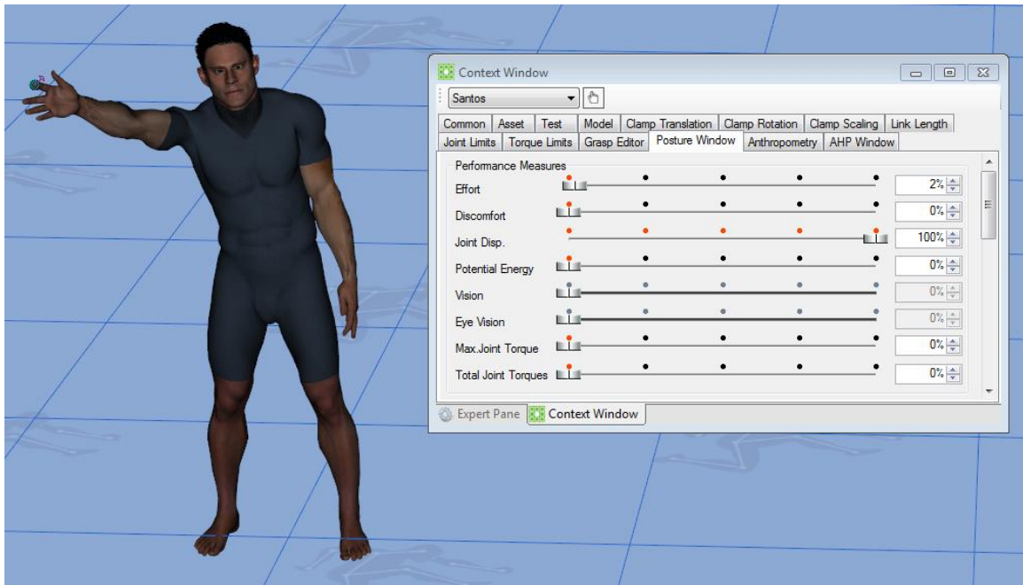
Figure 2.2: The result of MOO-based posture prediction for the index finger acting as the end-effector and reaching a target point in space.
